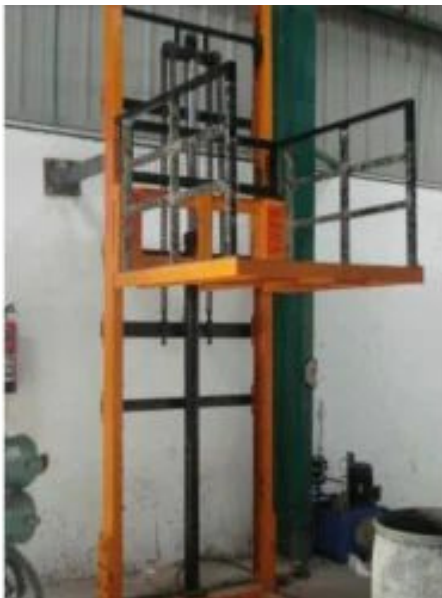
MS Goods Elevator
